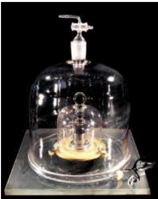
Fig. 1. The International Prototype of the Kilogram, or: An allegory of conflicting norms. The Kilogram has to be stable (protection by the bell jars) and accessible (the grip tongs). Reproduced by permission of the BIPM. All rights reserved.
